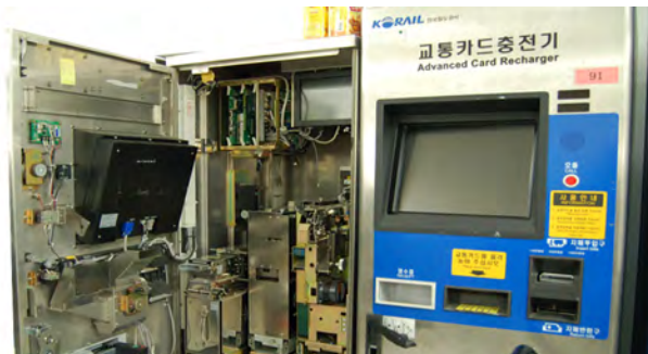
DFI's COM Express board is one of the four boards placed inside Korail's TVM.
